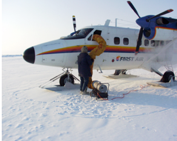
Photo 2: View of the forward Twin Otter aircraft set-up for hydrographic sampling, April, 2001. Co-Pilot Kevin Heslop placing ducting from Hermann Nelson heating unit through cockpit window.
